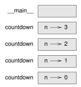
Figure 5.1: Stack diagram.
